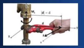
(Force vector,  $\mathbf{F}$ )× (moment arm d)  $\rightarrow$  Rotation of the pipe (amount and direction of rotation about z-axis)-a vector Vectors on x-y plane
