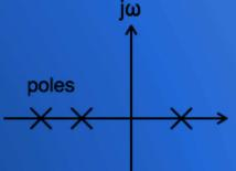
A system is said to be marginally stable when at least one pole of its transfer function lies on the jω axis of s-plane.
