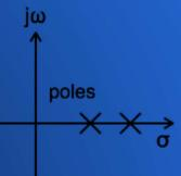
A system is said to be stable when all poles of its transfer function lay on the left half of s-plane.
