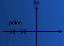
A system is said to be unstable when at least one pole of its transfer function is shifted to the right half of s-plane.
