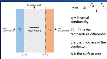
Thermal conductance is defined as kA/L and is measured in watts per degree Kelvin.
